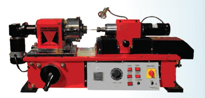
The machine is designed and developed for working of reduction and bearing portions of the Tungsten Carbide dies. Also the machine can be used for working special tools, extruder dies, round bores of hard metals etc.
