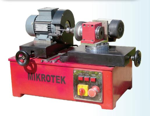
The Grinder is designed and developed for grinding accurate angles with  $\pm~0.5$  degrees on hardend steel and special wooden needles. The Machine mainly consists of a grinding wheel and reciprocating needle holding device. This grinder is used in combination with TC & Diamond die working equipment to achieve accurate die angles.
